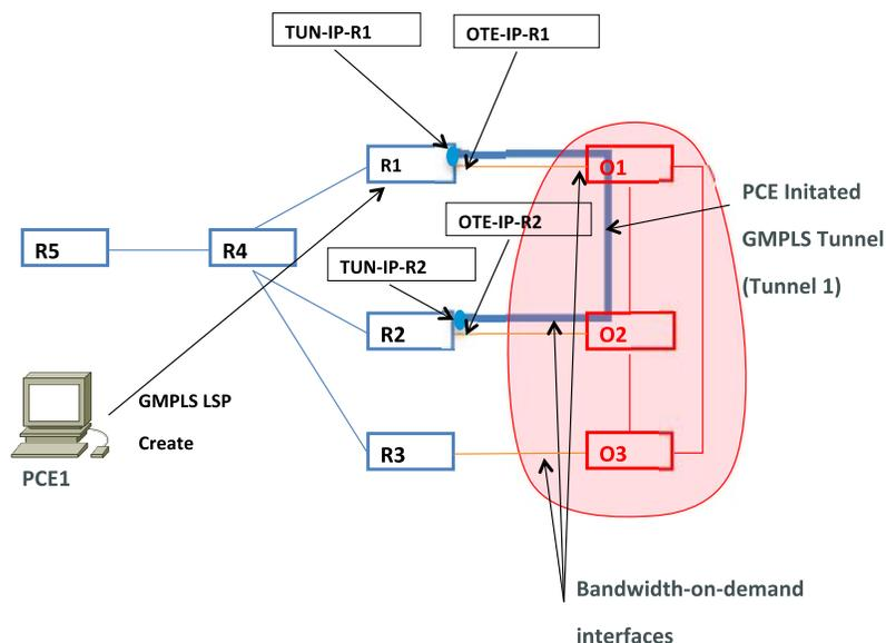
Figure 2. Use case higher-layer signaling trigger
